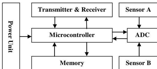
Figure 1: Wireless Sensor Node
